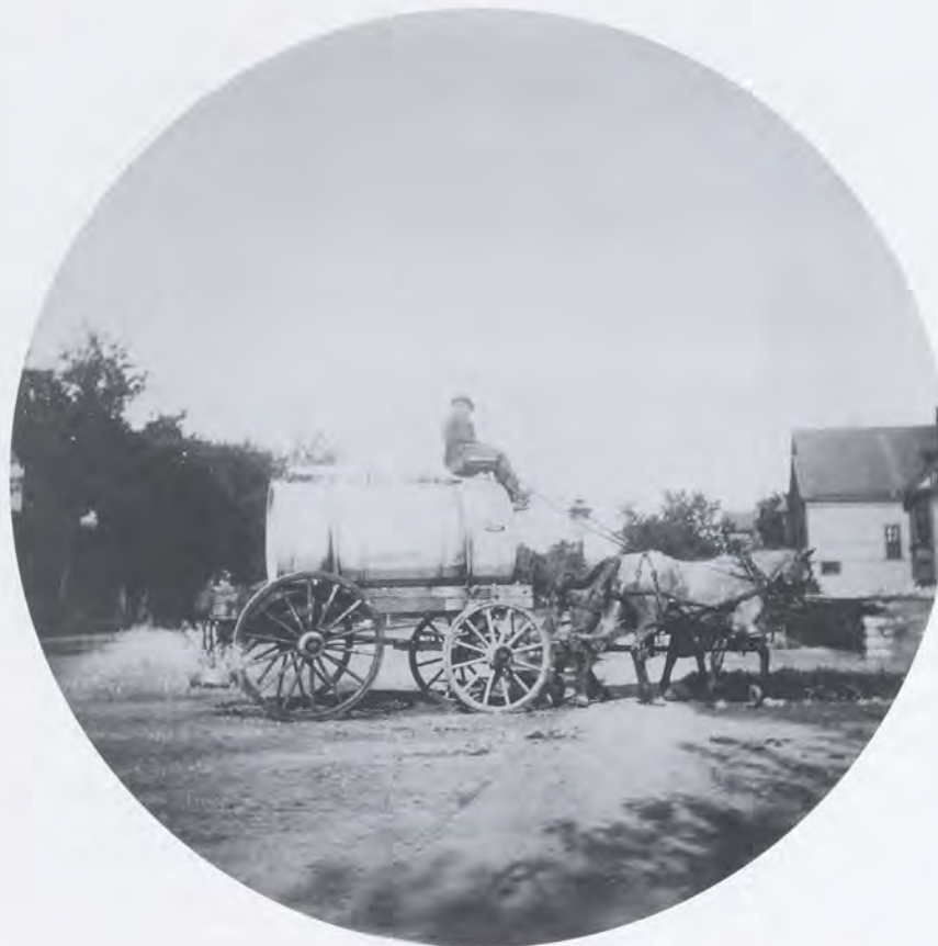
Water Sprinkling Wagon, probably in St. Paul, about 1885. By 1887 streets were being sprinkled to keep down the dust.
