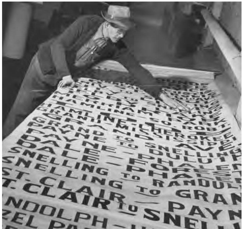
Snelling shop worker and destination sign roll. TCRT's Snelling Shops made everything from streetcars to destination signs. Minnesota Transportation Museum Collection.
