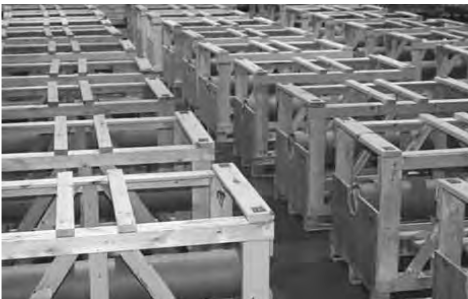
Members of the Industrial Division of Villaume specially designed these wooden crates for a customer who needed to ship a delicate, high-tech piece of equipment overseas. Each crate is built so that the customer’s product rests in the tube that runs the length of the center of the crate.
