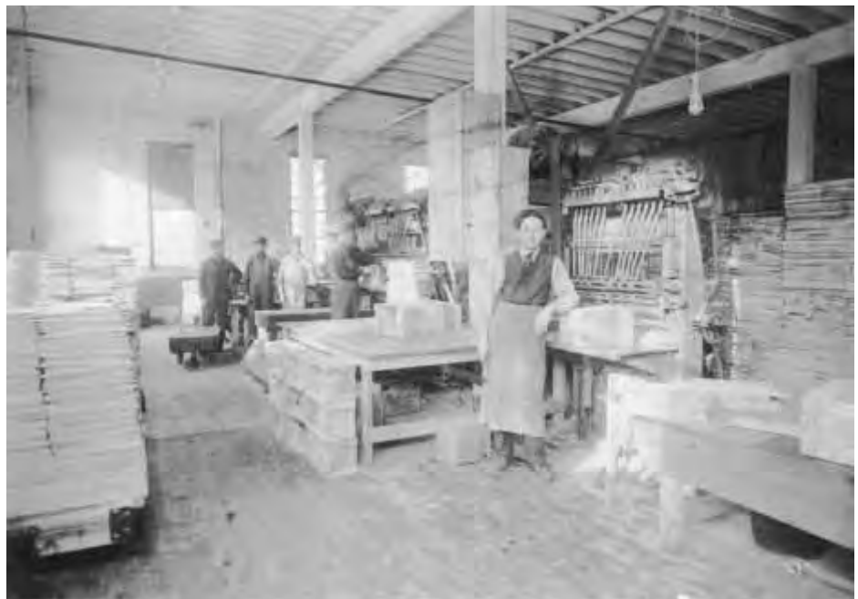
The saws and lathes that these men operated at the Villaume plant around 1900 were driven by a steam engine that transferred its power to each piece of equipment by a system of belts and pulleys. As the hanging light bulbs indicate, the plant also had electrical power for lighting.
