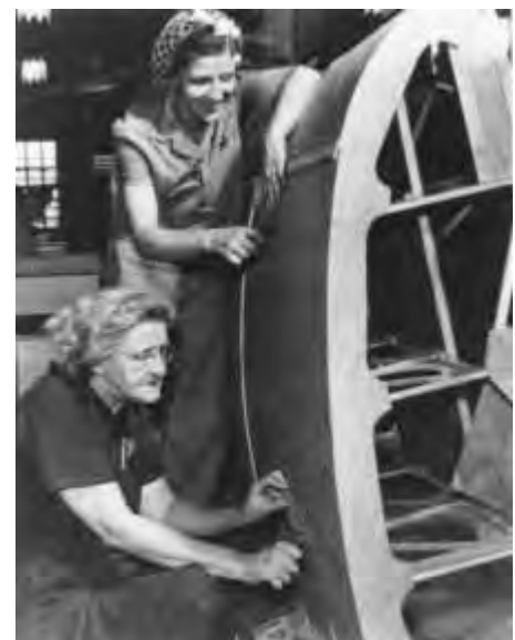
These women are doing some of the extensive handwork that was required for making the wings of a CG-4A glider at the Villaume plant.
