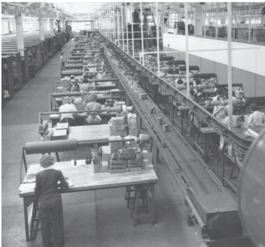
Special machinery and materials handling equipment needed to be installed for the Pratt & Whitney engine project. This photo shows the storage bins for parts on the left and the moving assembly line in the middle of two rows of worktables. Women workers faced each other at the tables while assembling parts. Photo courtesy of Brian McMahon.
