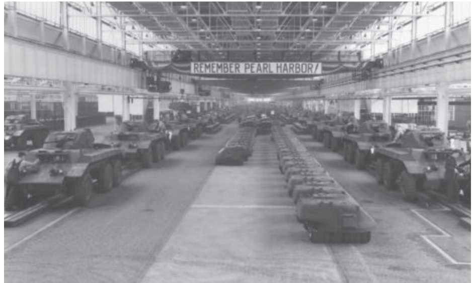
This photo was taken on the first anniversary of the attack on Pearl Harbor, December 7, 1942. It shows long lines of M-8s nearing completion in the crane bay of the plant. The overhead moving crane is dropping a turret on the body of an armored car in the left-hand row. Other turrets that are ready for mounting line the center of the bay. The crane was operated by a worker who is visible in a control booth on the upper left. Photo courtesy of Brian McMahon.
