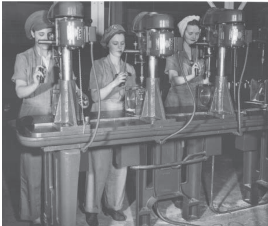
Three women operating industrial drill presses work on the pump machine that was a part of the Pratt & Whitney airplane engine. Note the employee badges with photo IDs pinned to their overalls. Photo courtesy of Brian McMahon.
