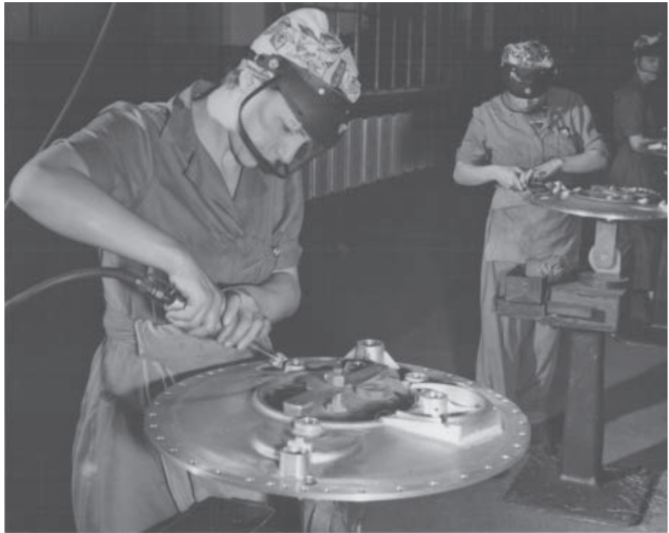
Two women sand cam supports for a Pratt & Whitney engine, wearing protective shields. Most women working on machinery also wore head scarves or hats, apparently of their own selection. Photo courtesy of Brian McMahon.
