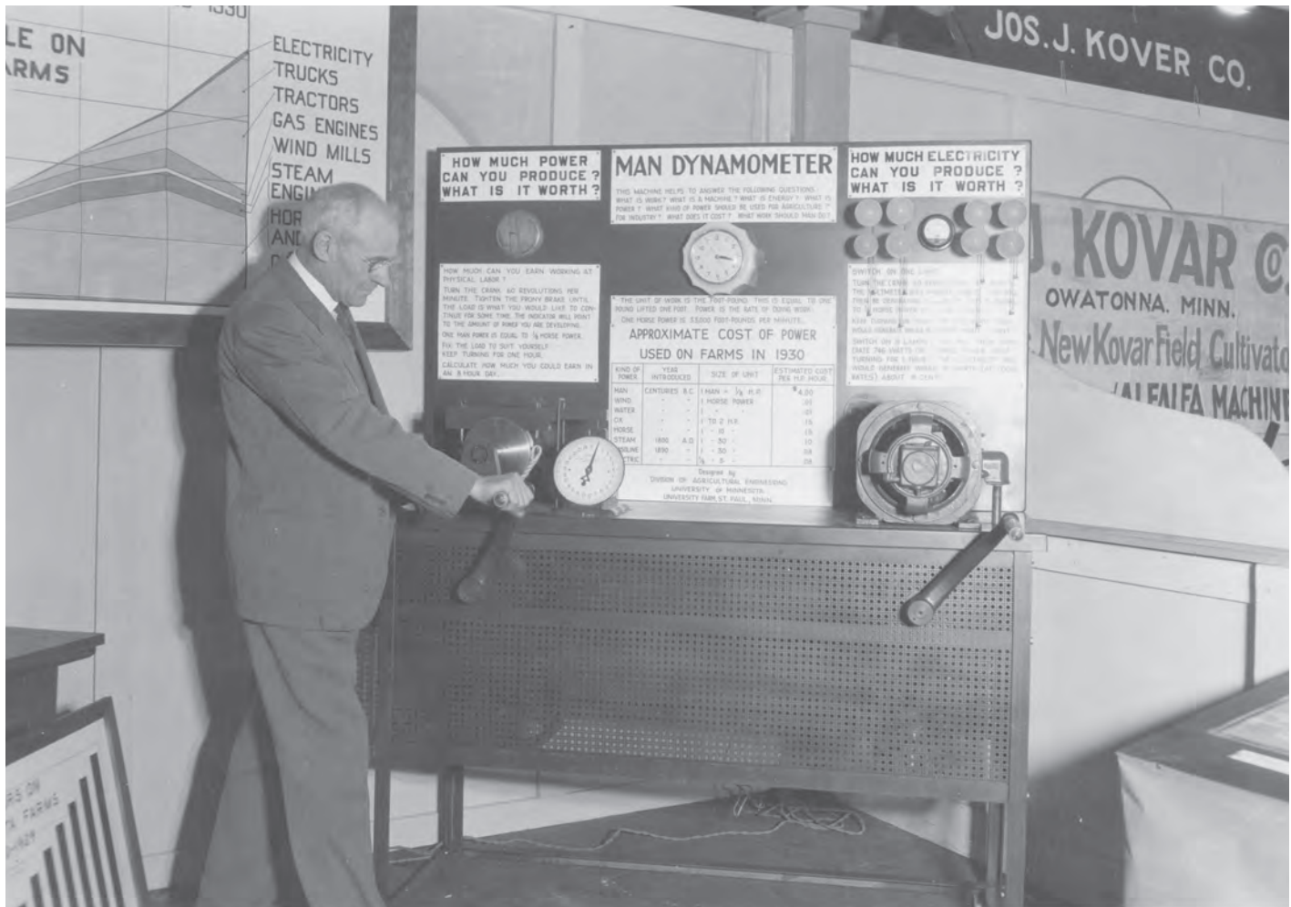
Here William Boss demonstrates his Man Dynamometer device that he developed in the early 1930s to compare the estimated cost per horsepower per hour of power on farms depending on its source: human, wind, water, oxen, horse, steam, gasoline, and electricity. Boss Family and Business Collection. Photo courtesy of the Minnesota Historical Society.
