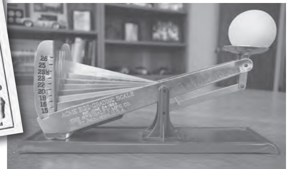
An advertisement from a 1933 issue of Poultry Supply Dealer magazine for an Acme Egg Weighing Scale manufactured by SMC beside an example of the scale in the SMC collection. The advertisement is from the Boss Family and Business Collection, Minnesota Historical Society. The photo of the Egg Scale is courtesy of the Specialty Manufacturing Company.
