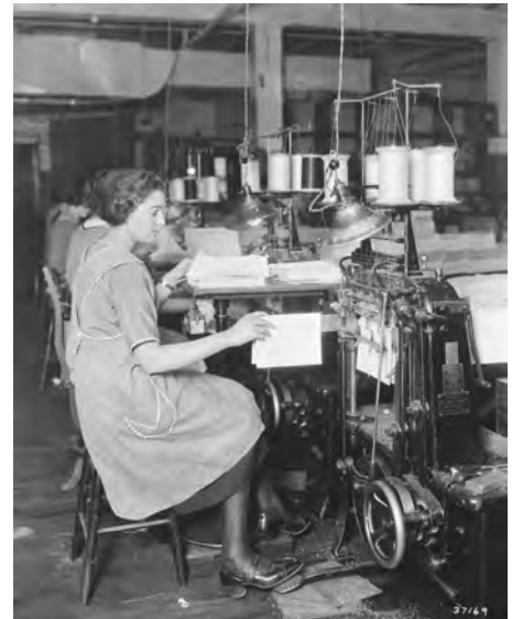
Once signatures for a law book from West had been printed and folded, women in the stitching department operated sewing machines, such as the ones seen here, which sewed each printed signature into a book block to which a cover was then glued. By varying the colors of the spools of thread used in sewing, each machine could be identified and the quality of the work of its operator evaluated. Photo courtesy of Thomson Reuters.
