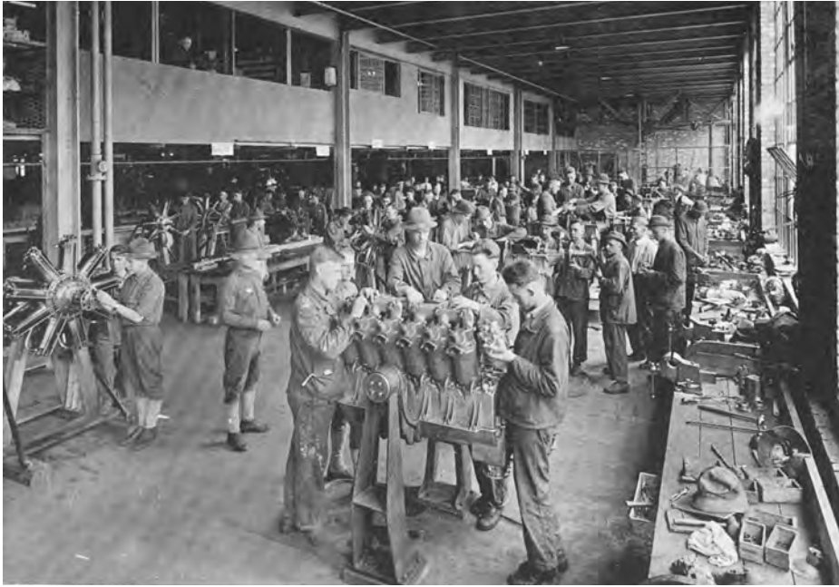
Students learned to tear down and repair aircraft engines, including the Liberty, the engine specifically developed to power the American air fleet.
