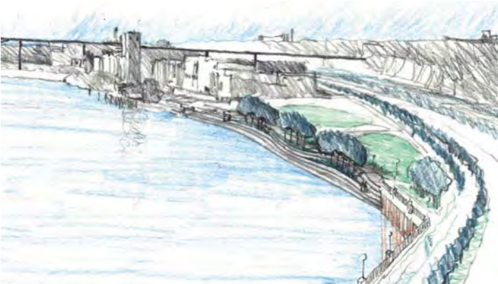
East side River edge in the future: Over time, replace riprap as part of ongoing maintenance operations with terraced stone or large concrete blocks to allow River access and infill plantings protected from River scour.
