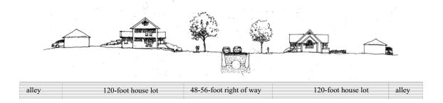
Figure 10.10 Local/Residential Street—Leaky Pipe with Curb and Gutter
