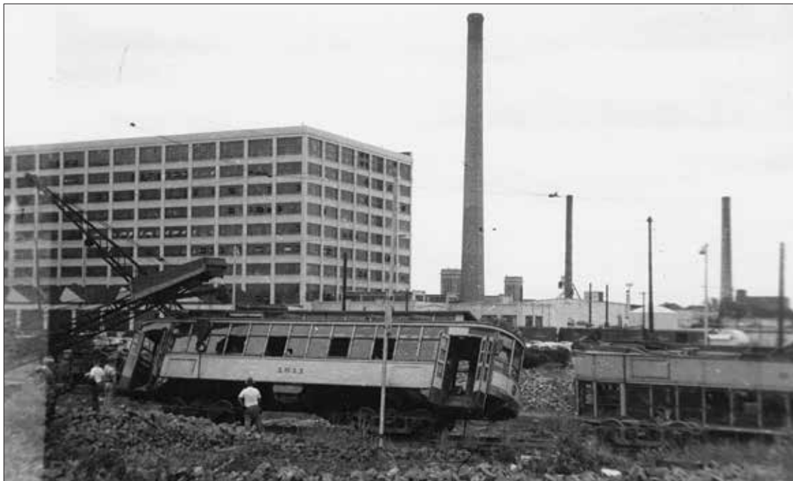
In 1954, forty-two years after it was new and left the Snelling Shops, car 1511 returns to Snelling for its funeral. Once workers finish tipping it on its side, it will be set ablaze. When the immolation is complete, its metal remains will be sold for scrap. In the background is the massive warehouse that was once a part of the Montgomery Ward facilities on University. Photo courtesy of the Minnesota Historical Society.
